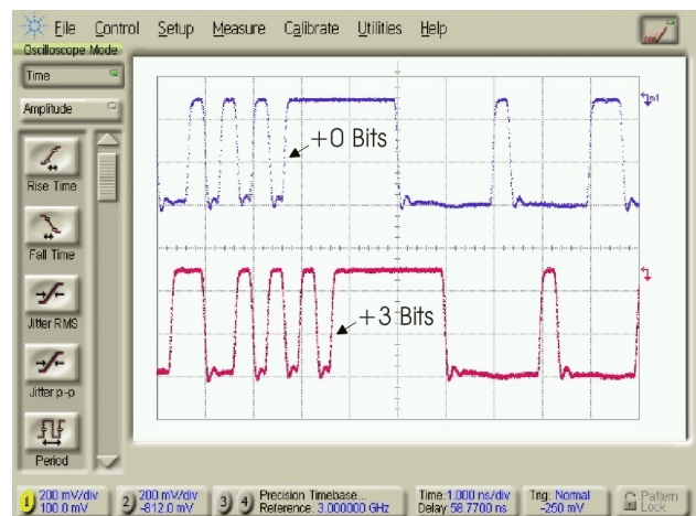
Figure 3: Example of a PRBS signal delayed by 3 bits
